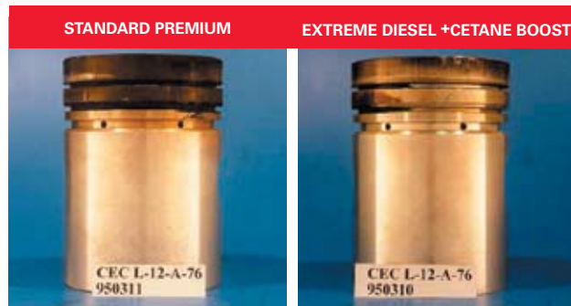
Comparison of piston cleanliness using a standard premium diesel fuel versus diesel fuel treated with Extreme Diesel +Cetane Boost. Test Method: MWM-B CEC L-12-A-76
